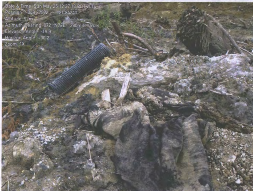
Figure 5.2.33 Drainage pipe and filter fabric from SR 530 transported to the southwest by initial debris flow. Camera position: 48.27572°N, 121.84240°W, view looking east-southeast.
