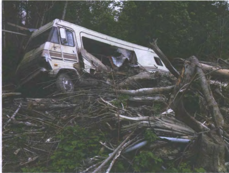
Figure 5.2.28 Recreational vehicle (RV) at the distal edge of the flow. Image shows damage to its side by a root-wad that is still present beside the vehicle. There is little evidence of earth debris: the RV was pushed and damaged by woody debris, as if carried by a flood. Camera position: 48.27528, -121.84160.
