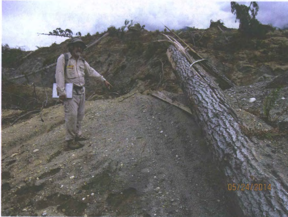
Figure 5.2.10c. pair of track-like impressions in the loose sand indicate that the log impacted violently and bounced before coming to rest. Photo taken by GEER on May 24, 2014. Camera position: 48.281458°N, 121.848316°W, view south.
