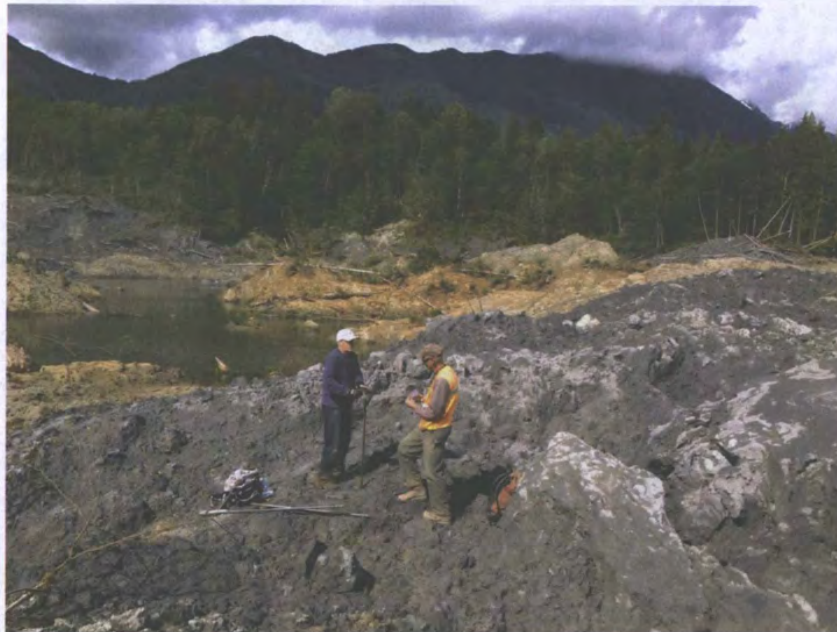
Figure 5.2.15: Hand auger boring (HA-3) into lacustrine material on the northern margin of Zone D. Camera location: 48.28118, -121.84519; view to northeast.
