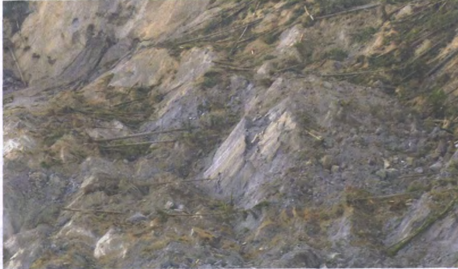
Figure 5.2.10a. Oblique view of two approximately 100-ft-long (30 m) fallen trees (near the center of the image) that have been dragged downslope after they were felled. They indicate the extension in this part of the slide mass. Photo by Eric Jensen, King County Sheriff Department, photo date 3/24/2014.
